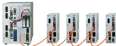
YC-LINK couples single-axis controllers to a 4-axis controller
