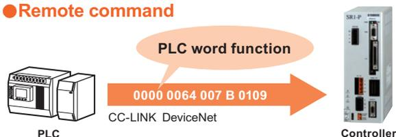
This uses CC Link or DeviceNet word functions to issue various data or commands to the robot. It makes full use of word function expandability ranging from simple operation instructions to writing of point data and other sophisticated instructions and allows fully and flexibly using robot controller functions from a host device.
