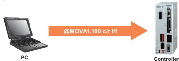
A PC connected via RS232C or Ethernet <sup>Note</sup> can be used to issue various commands and data directly to the robot controller or receive data and status. All operations performed from a teaching pendant can be executed from a PC.
