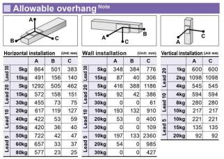
Note. Distance from center of slider top to center of gravity of object being carried at a guide service
